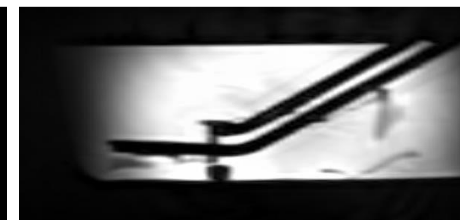
Figure 4: T2-weighted image of water phantom showing no apparent signal from the marker.
