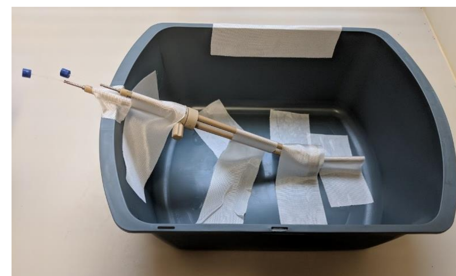
Figure 1: Water phantom set-up with plastic ring HDR applicator and MRI-positive markers inserted.
