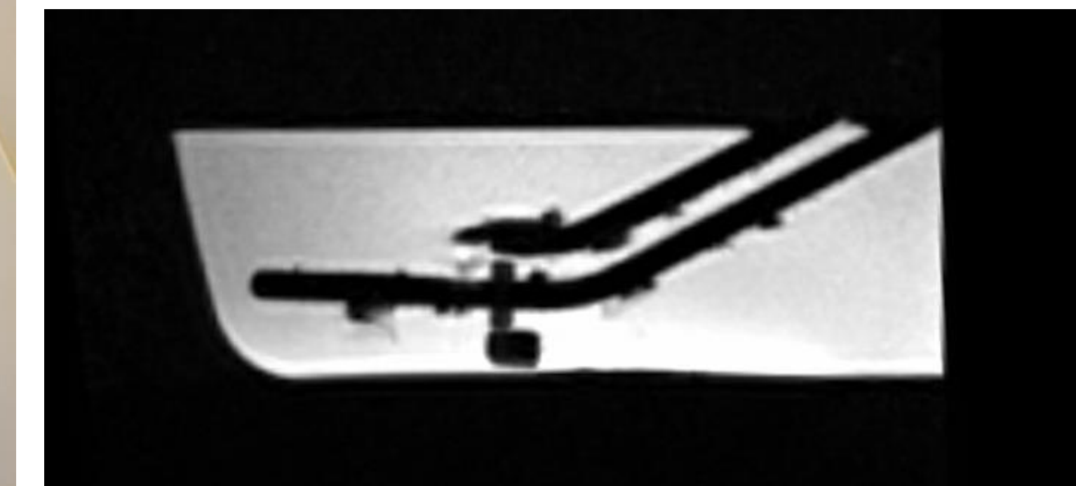
Figure 2: Negative contrast of HDR plastic applicator on T1-weighted MRI scan.
